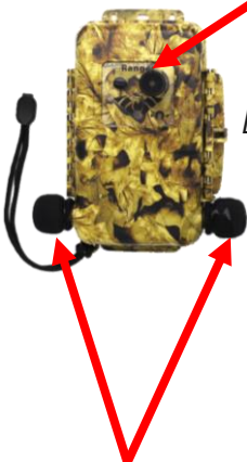
2 Microphones ultrason (10 – 150 kHz)
