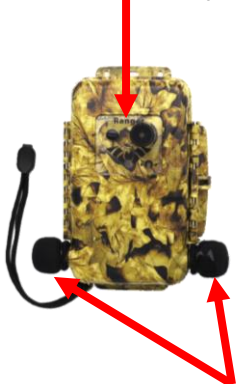
2 Microphones ultrason (10 – 150 kHz)
